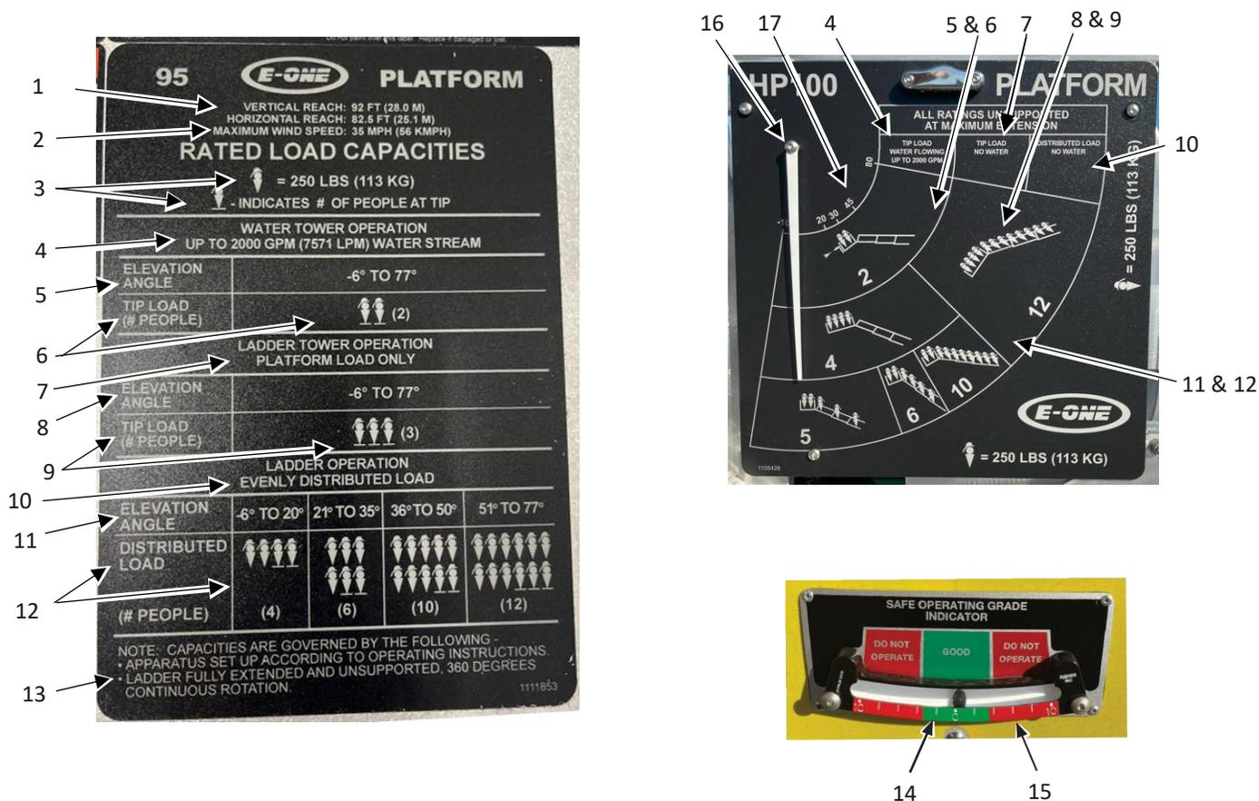
Sample Load Chart, Inclinometer, & Level Indicator
