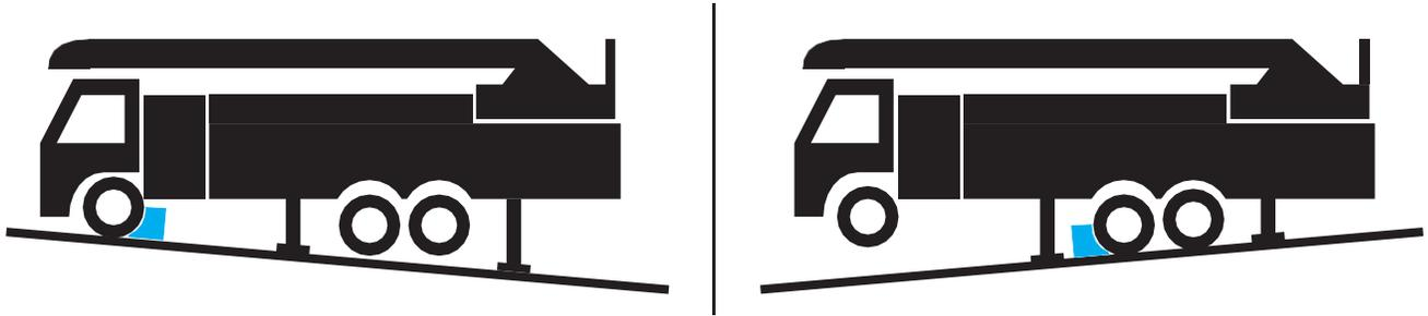
Leveling an Apparatus with 4 Stabilizers
