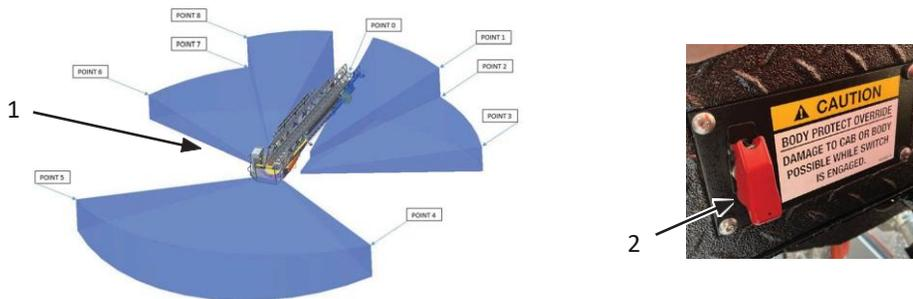
*Ladder Movement Stops Prior to contacting Body of Apparatus*
