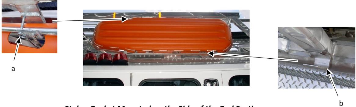
**Stokes Basket Mounted on the Side of the Bed Section**
