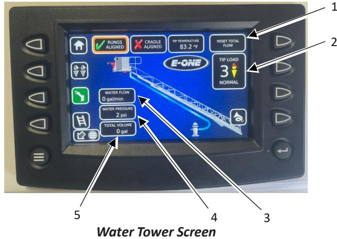
1. **Reset Total Flow** – Allows you to reset the Supply Water Flow indicator to zero (0).
