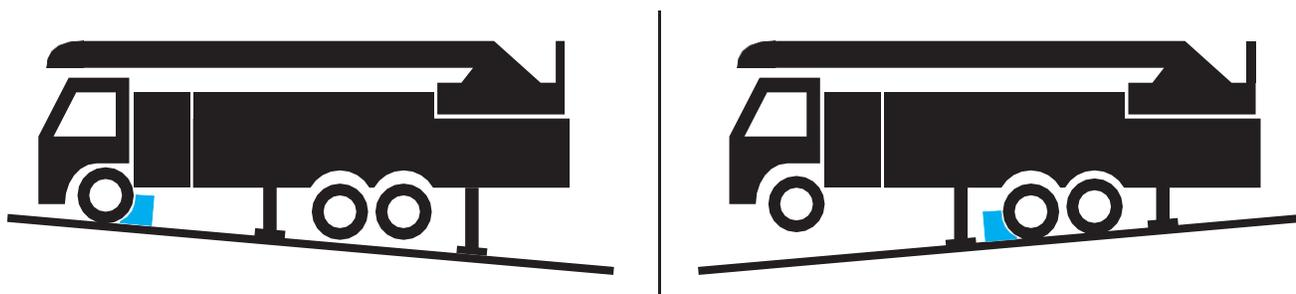
Leveling an Apparatus with 4 Stabilizers
