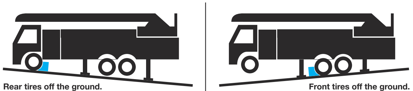
Figure 4-5. Leveling an Apparatus with 4 Stabilizers
