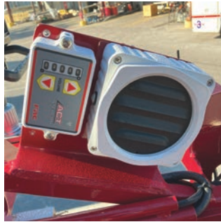
Figure 3-31. Ladder Tip Communications System
