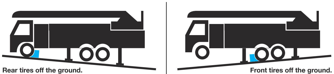
Figure 4-4. Leveling an Apparatus with 4 Stabilizers
