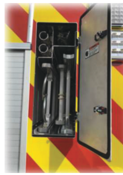
24-ft 2-section; 14-ft roof; attic; and (2) pike poles stored in the body.
