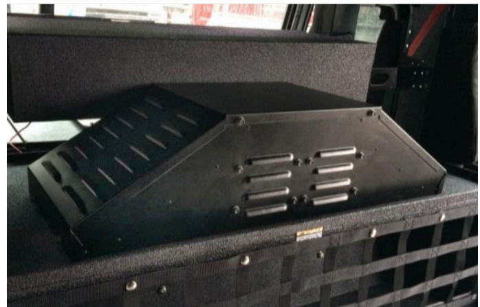
HEPA filtration system for cab interior
