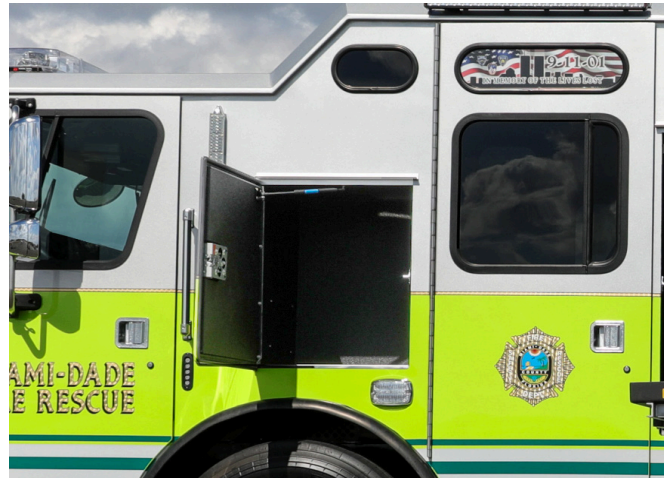
Over wheel bunker gear storage (exterior access only)
