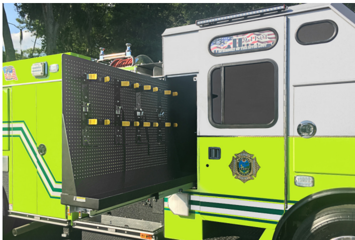
Pull-out SCBA mounting board isolated from cab interior
