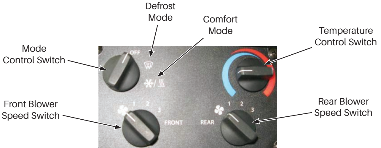
Figure 3-50. Single Overhead HVAC System
