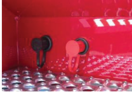
Figure 5-26. Battery Jumper Terminals
