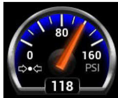
Figure 3-16. Auxiliary Air Pressure
