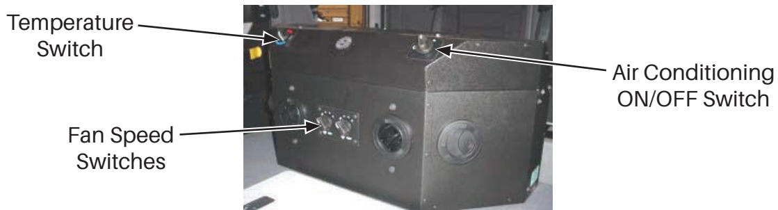
Figure 3-53. Tunnel Mounted HVAC System
