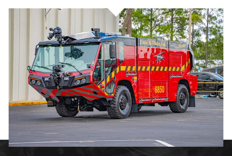
The E-ONE TITAN  $4\times4$  AT (Air Transportable) Series is designed as an aircraft rescue firefighting vehicle that allows transport on C5, C17, and C130 aircraft. On and off-road capabilities allow the vehicle to respond in a timely manner to aircraft accident sites across terrain which might otherwise be inaccessible to other standard fire apparatus.
