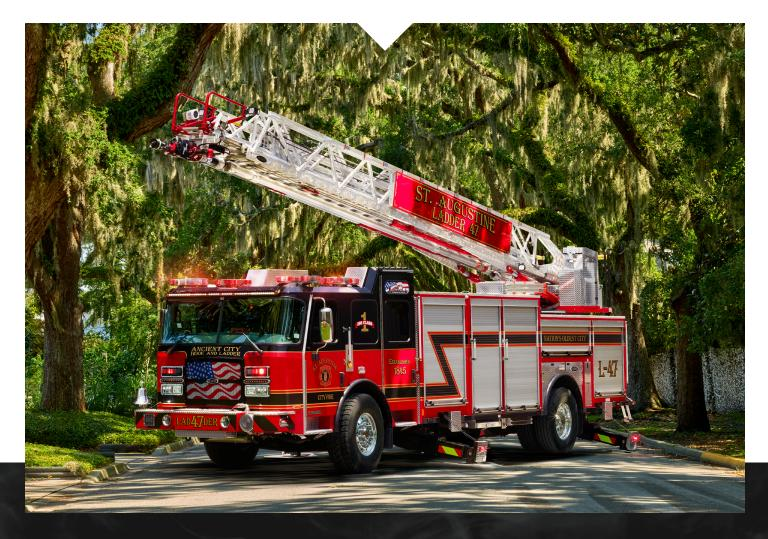
The Metro 100 Quint is a single axle aerial with 100' of vertical reach and up to 92' of horizontal reach with a pump, tank and hose bed. The crisscross underslung outrigger spread of only 11' allows for set up in tight locations.
